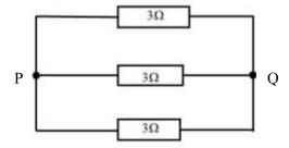
So the equivalent circuit is simply three,  $3\Omega$  resistors in parallel, so the equivalent resistance is  $1\Omega$ .
