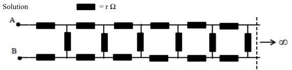
The above diagram shows an infinite "ladder" of resistors of value r  $\Omega$  each. If we were to cut at the broken line we would get two pieces as shown: piece R to the right and piece L to the left
