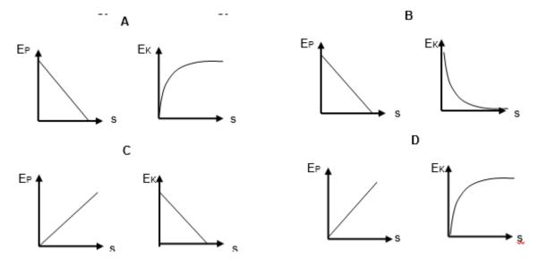
As the ball-bearing falls in the oil, its speed will increase in such a way that the downward acceleration will decrease and eventually be zero, and it will continue at a constant speed, known as its "terminal velocity" until it reaches the bottom of the cylinder. This means that the kinetic energy will increase to a steady maximum. The potential energy will simply decrease linearly with distance.
