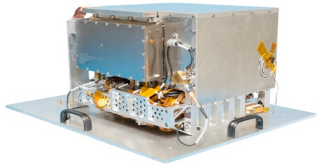
NASA is currently working on the Deep Space Atomic Clock set to launch in 2016. The miniaturized, ultra-precise mercury-ion atomic clock is far more stable than today's best navigation clocks and will greatly improve future space navigation. Credit: NASA/JPL
