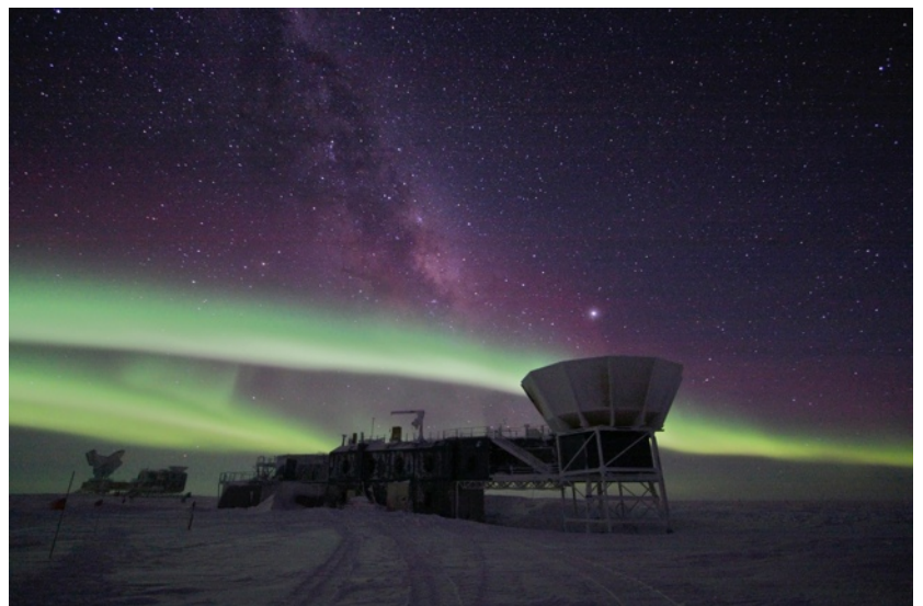
FIGURE 1: BICEP2 at South Pole. BICEP2 is a 26 cm CMB telescope with 500 highly sensitive bolometric detectors situated at the South Pole, a location ideally suited for minimizing atmospheric interference because of the low water vapor column density there. In March 2014 the BICEP2 team announced having discovered primordial gravitational waves from inflation with a tensor-to-scalar ratio of r = 0.20^{+0.07}_{-0.05} . Subsequent analysis, however, cast doubt on this claim on account of an underestimation of the contribution of the polarized emission from interstellar dust in our own galaxy. BICEP2 mapped a small patch of the sky in a microwave band centered around 150 GHz. (Credit: Keith Vanderlinde).
