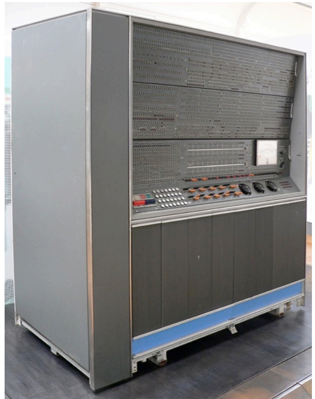
Comment by the editor: The Atomic Weapons Research Establishment (AWRE) at Aldermaston used an IBM 7030 (picture, Copyright © 2006 David Monniaux), also known as Stretch. The price of this first transistorised supercomputer of IBM in 1960 amounted to $13.5 Million.
