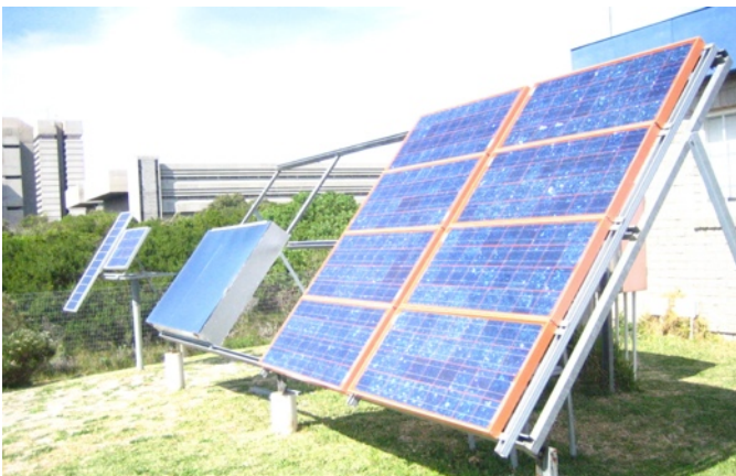
Rack with multicrystalline silicon modules and heat box
